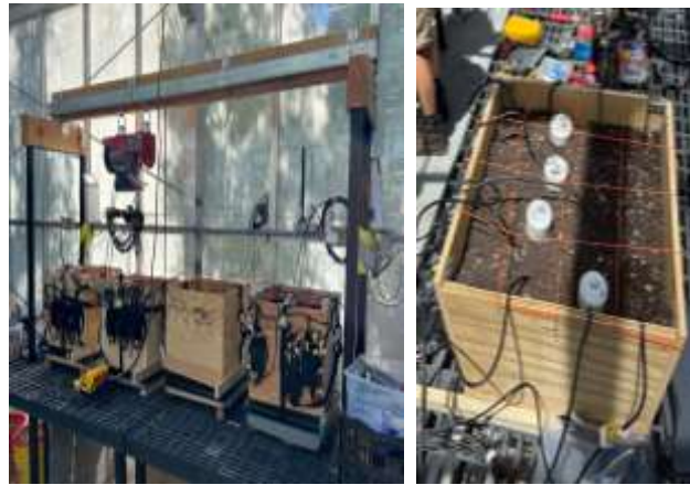
Figure 1. Data collection setup. The picture on the right shows the sensor layout of a box.
