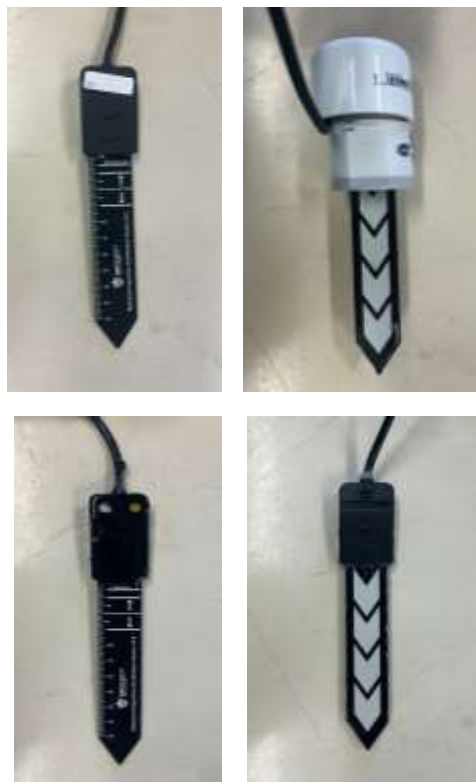
Figure 2. Sensor protection treatments. Upper left: Unprotected sensor, Upper right: Epoxy coated sensor, Lower left: Epoxy drenched sensor, Lower right: Glued sensor
